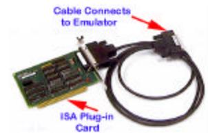
**EPC - LPTx printer port** Emulator Parallel Cable which communicates with the pod through a standard PC parallel port (LPTx).
