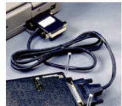
**USB Interface** The new USB interface is available now. This cable connects to the USB connector on the appropriately equipped PC and to the emulator with the standard 25-pin D shell connector. This cable will work with all Windows versions that support USB and such as Windows 98 and 2000Pro/XP.
