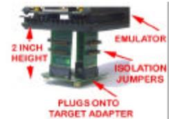
**Extender board** This board fits between the pod and the adapter to give additional clearance between the pod and the target. It raises the pod an additional 0.50" (12.7mm) above the target. It does not support the 10-pin XBUS connector (JP46) used by some Xperipheral daughtercards.
